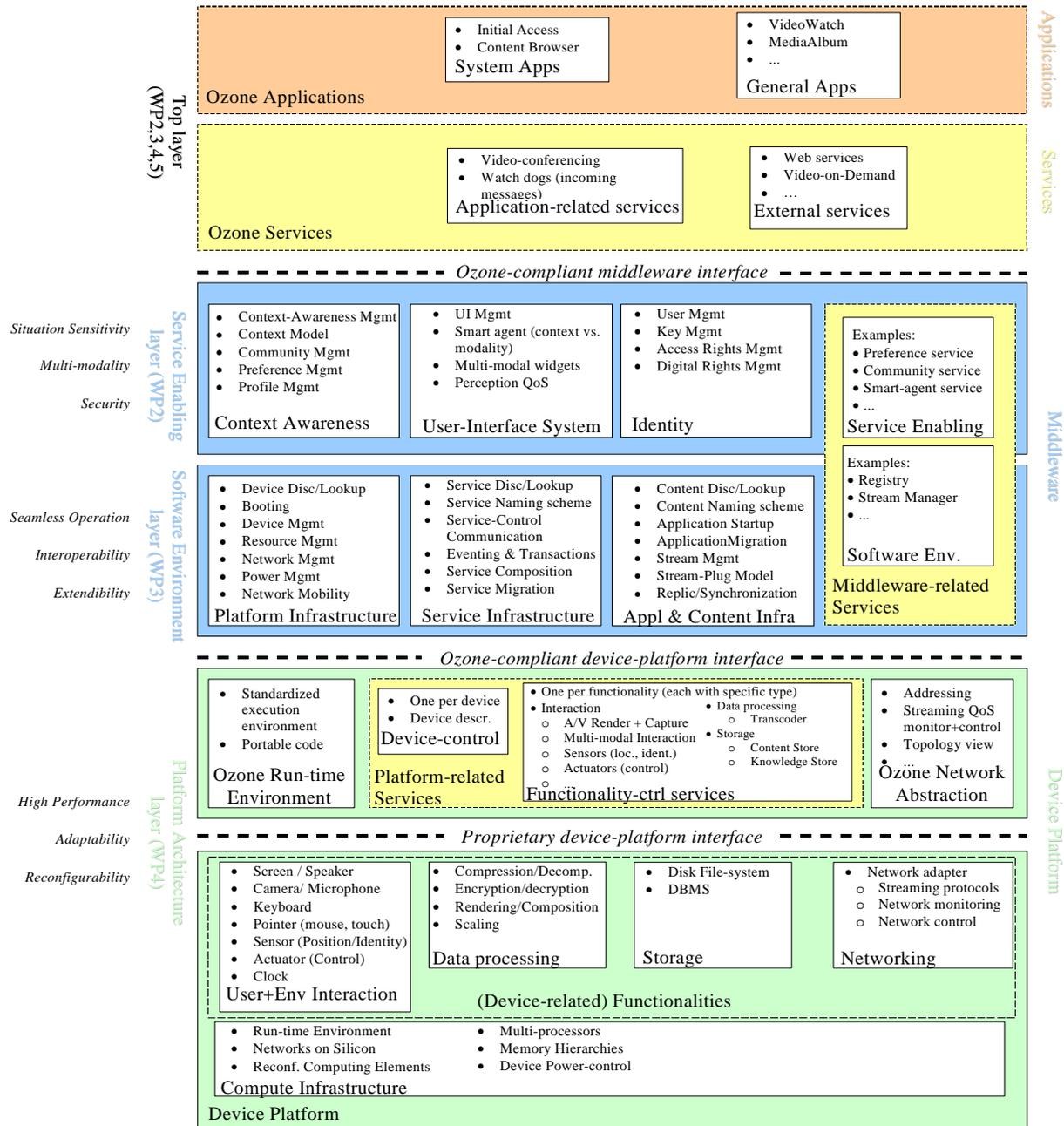
Figure 5.4 Ozone device architecture – a layered functional decomposition.
