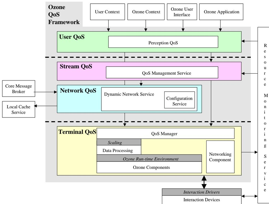
Figure 5. 6 QoS view of the Ozone architecture.
