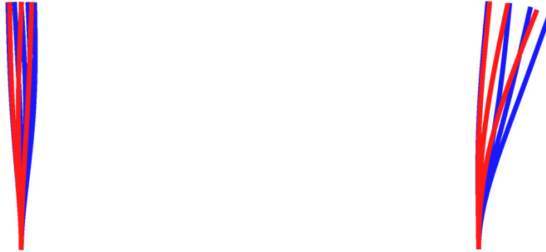
Figure 5: The forward (blue) and backward (red) stroke of a cilium in a Newtonian fluid (left) and the shear-thinning fluid (right). Both have the same actuation cycle with f_1 = 4 \cdot 10^5 N/m 3 .
