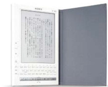
Figure 3: Sony LIBRIé e-Book Reader this chapter, E Ink supplies electronic ink for this product. Toppan Printing process the ink into a thin optical film and Philips adds the driving electronics component. The solution has then been adopted in the Sony e-Book reader "LIBRIé".
