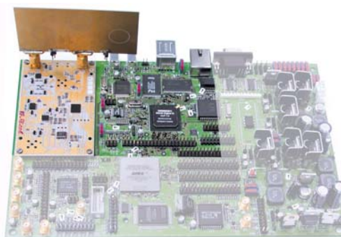
Development board with Thomson's HiperLAN2 chipset
