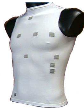
Figure 1. MyHeart instrumented shirt - skin layer; Textile electrodes are clearly visible on this under layer of the garment
