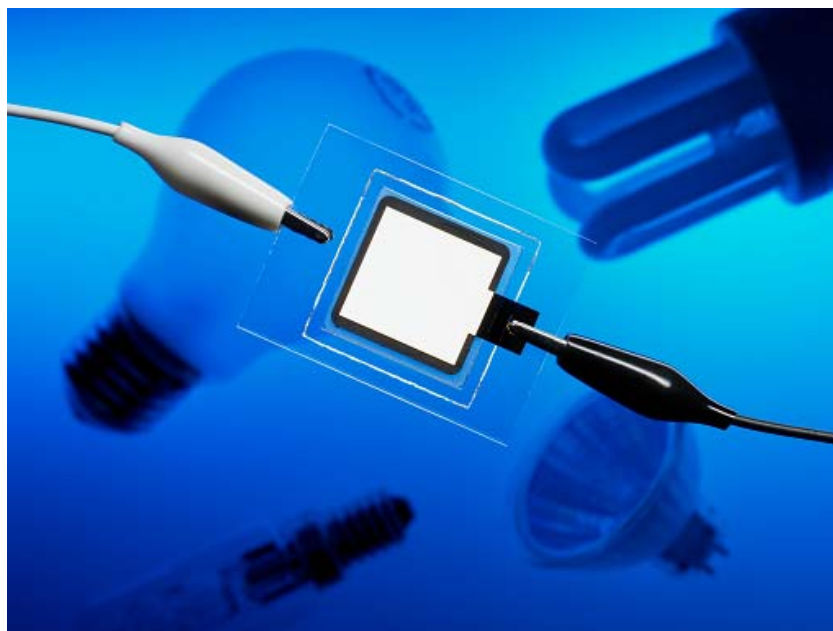
Figure 3.6: Picture of the two color fluorescent white p-i-n OLED produced at Novaled.
