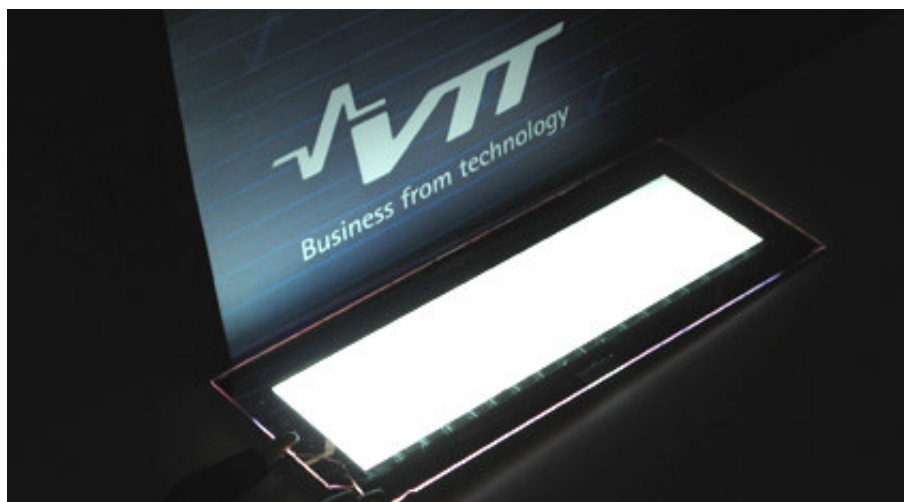
A white gravure printed OLED device (source VTT)
