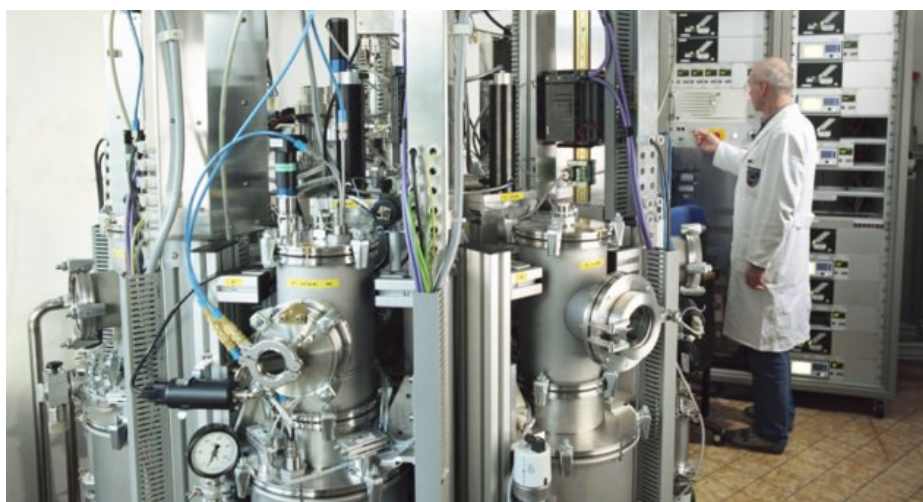
Small Molecule OLED deposition under high vacuum (source Philips)
