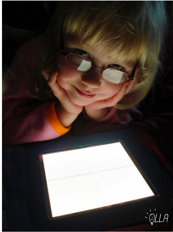
Caption: OLED is a revolutionary novel efficient lighting technology. The thin glass plate lighting tiles are based on organic materials and do not make use of mercury. Therefore OLEDs are (potentially) fully recyclable. (Picture source: the OLLA project / Philips Lighting)
