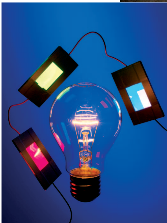
Fig. 1: Monochrome OLEDs have already surpassed the efficiency of the light bulb (Source: Novaled)
