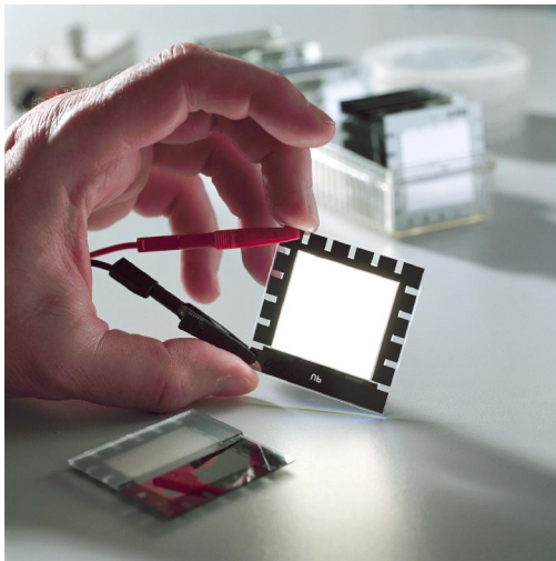
A warm white small molecule OLED research sample measuring 35 by 35 mm 2 . (Picture by Philips)
