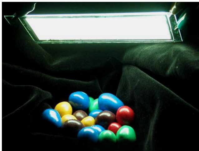
Lighting tile with 35 cm 2 active area using a white copolymer (Picture by Siemens)
