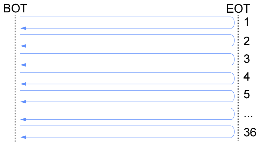
figure 5: MLR1 tape partitioning
