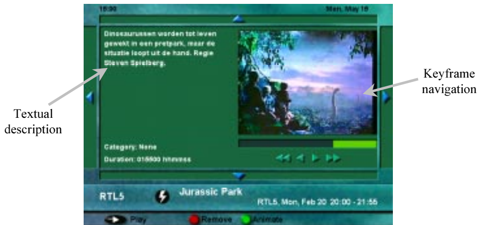
Figure 16: User interface screen displaying information on a selected recorded program, including a textual description from the EPG, and key-frames for quick browsing or navigation.
