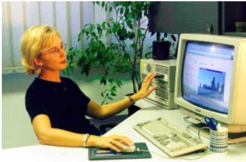
Figure 20: WEB-VCR demonstrator featuring the VCR like Interface playing a video stream from the Internet while a tape is being inserted in the Combo System for storing
