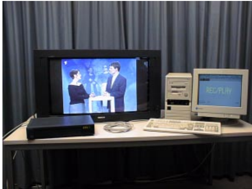
Figure 3: Demonstrator for IEEE 1394 based DVB/MPEG transmission
