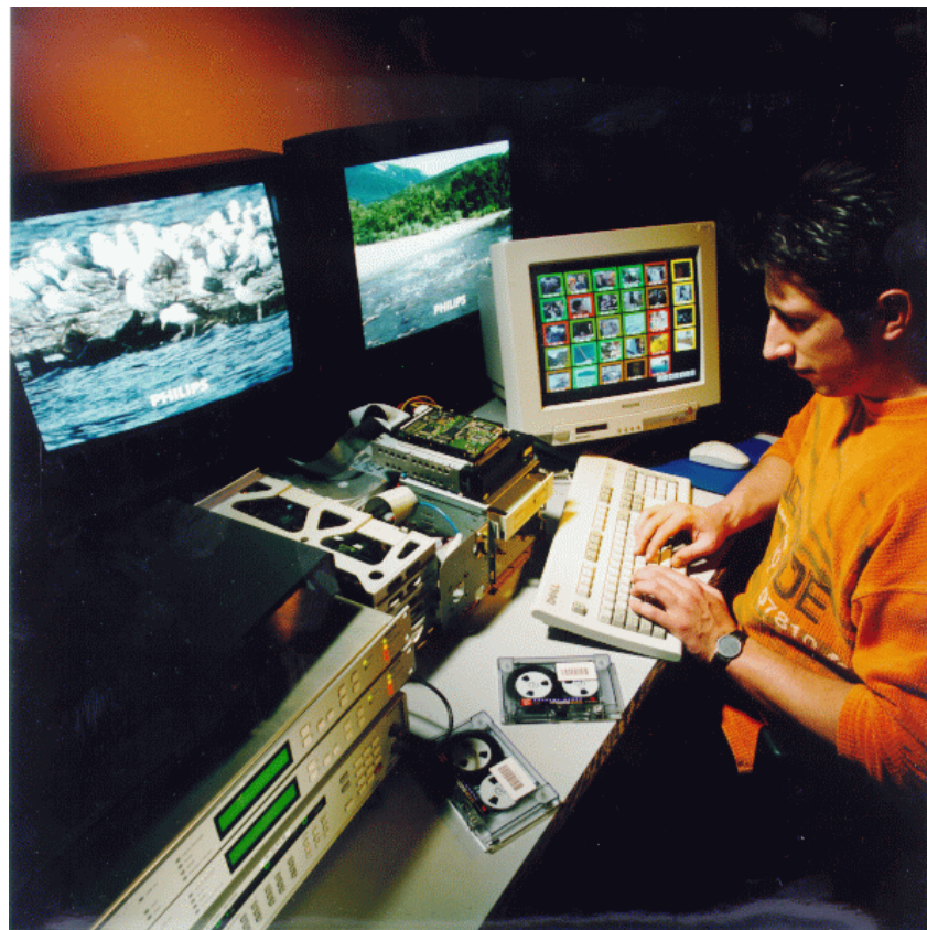
Figure 7: SMASH Combo server with settop boxes, tape and disk drives and a simple graphical user interface of the DVB-VCR demonstrator: The key-frames represent the contents of the tape.
