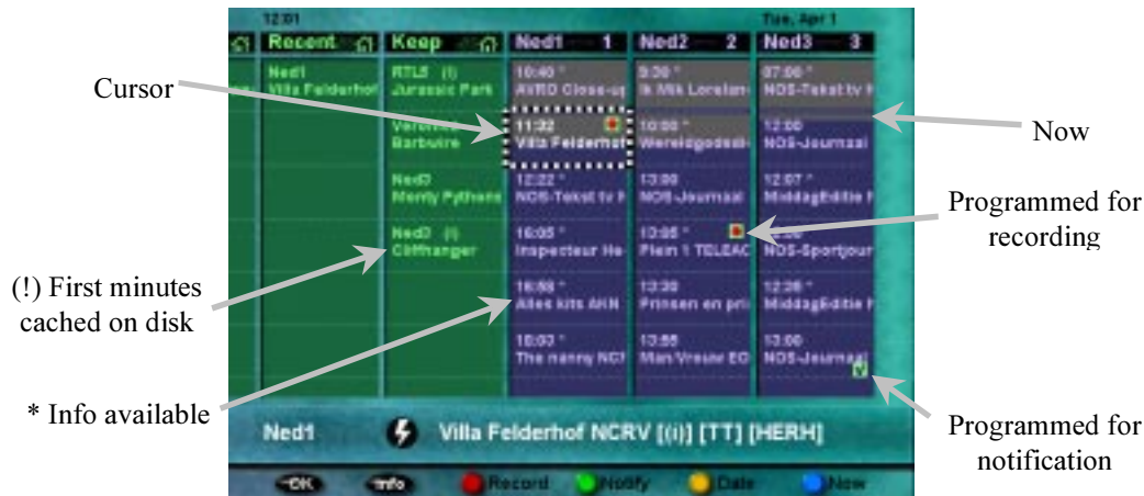
Figure 15: User interface screen displaying a combined table of contents and electronic program guide.
