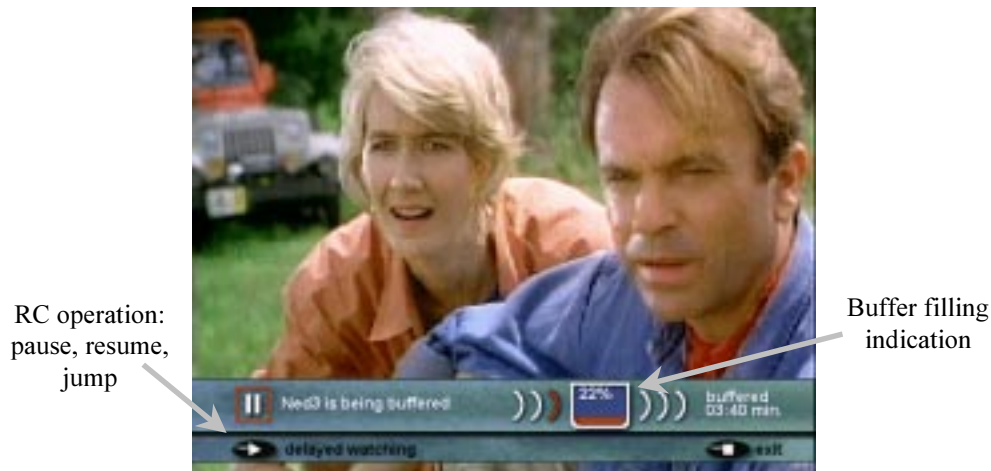
Figure 17: User interface screen displaying the pause button function. The video is frozen during a pause, and the buffer state is displayed.
